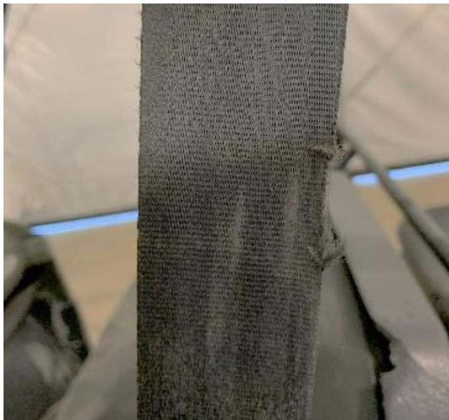
Figure 19 – Fraying on MV Seatbelt (Tab Z-29)
